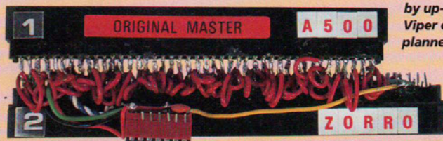
A Zorro bus. Now, can you spot which wire is connected wrongly?
